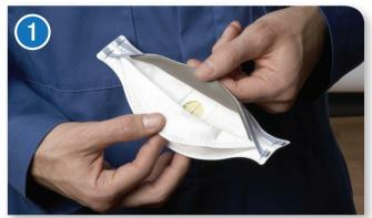
**1a.** With reverse side up separate top and bottom panels of the respirator. Bend slightly at the centre of the nose clip.
