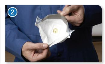
**1b.** Ensure both panels are fully unfolded to form a cup shape.
